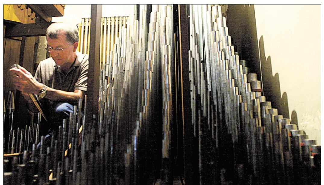
Restoring a pipe organ often means working in tight places. Organ builder and restorer Madison Lindsey sits between sets of pipes in one of the pipe chambers at First Presbyterian Church as he adjusts the sound quality of one of the pipes. Lindsey and Troy Scott of Laurel are making adjustments to complete an 18-month project, which will be celebrated with an organ recital May 23.
