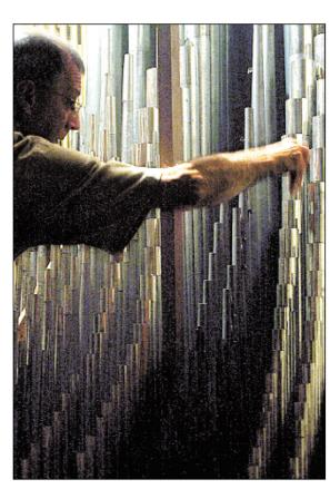
Madison Lindsey, above, reaches over several tiers of pipes to replace one that has been adusted for sound and tonal quality. To work on the pipes in all of the three chambers, Lindsey uses numerous tools, including various knives and an air pressure gauge. The tools are used to control the air in the pipes. Inset, all of the old leather valves, like the darker one at left, have deteriorated over time; they have been replaced with valves, such as the one at right, made of kangaroo leather.
